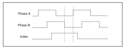
Figure 14. Encoder Signal Phasing, CW Rotation
